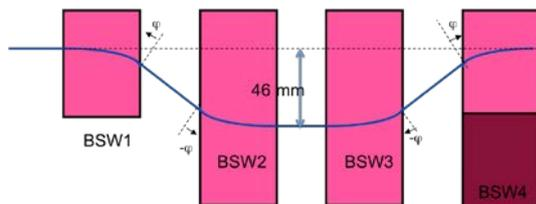
Fig. 3 Sketch of the injection chicane bump.
