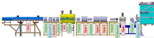
Fig. 1 Layout of the REX normal conducting linac. The seven RF structures are labeled in red.
