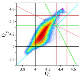
Fig.1 Space-charge tune spread at injection energy in the PSB and resonance lines in the tune diagram
