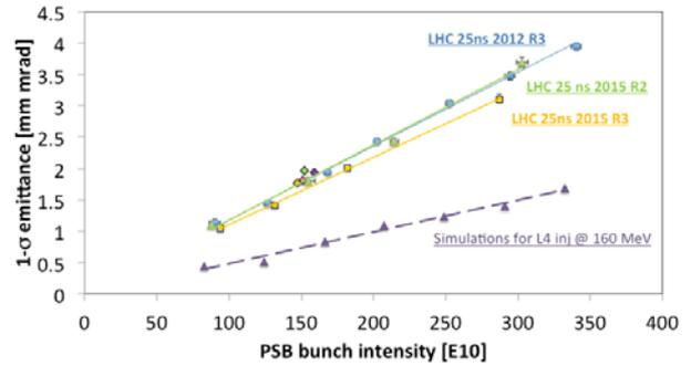
Fig.2 The measured optimized beam brightness and the simulated curve after the 160 MeV upgrade
