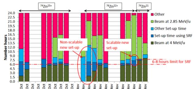
Fig. 3 Beam time available to users during the first HIE-ISOLDE physics experiment in green. Time spent setting up the machine in blue
