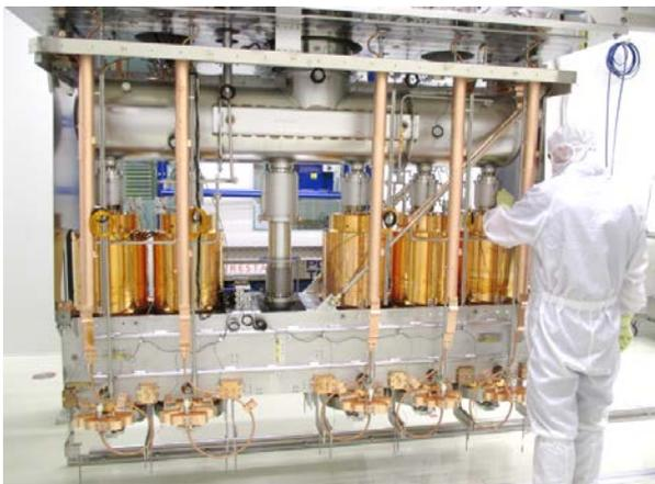
*Fig. 4 Final verifications on cryomodule 2 in the cleanroom in SM18 before closure and transport to the ISOLDE facility.*
