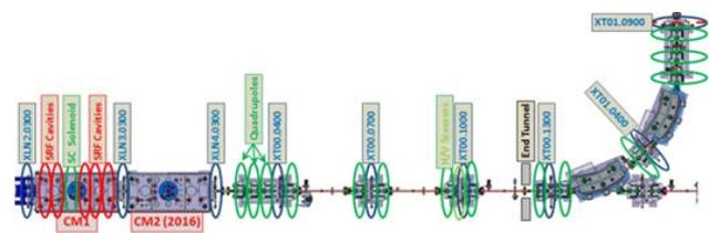
Fig. 2 Layout of Phase 1 of the HIE-ISOLDE linac and the first experimental line. The nine diagnostics boxes are labeled in blue.
